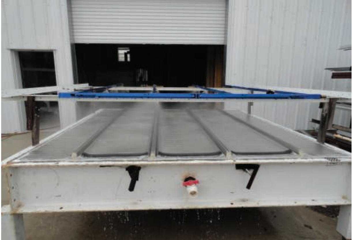
PANELS DURING WATER TEST
